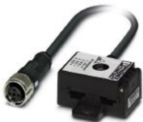
AS-Interface distributor with IP67 protection for two flat-ribbon conductors, with 2.0 m PUR round conductor and a molded, straight, A-coded, 4-pos. M12 SPEEDCON socket
