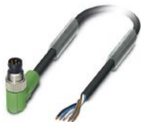
Sensor/actuator cable, 5-position, PUR halogen-free, black-gray RAL 7021, Plug angled M8, coding: B, on free cable end, cable length: 3 m
