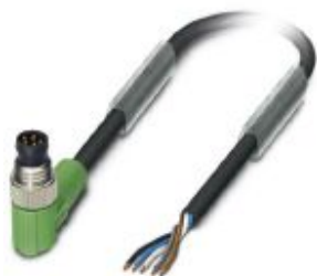
Sensor/actuator cable, 5-position, PUR halogen-free, black-gray RAL 7021, Plug angled M8, coding: B, on free cable end, cable length: 5 m
