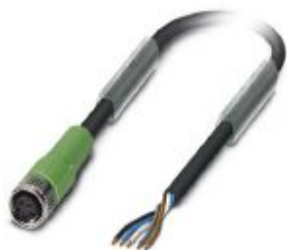
Sensor/actuator cable, 5-position, PUR halogen-free, black-gray RAL 7021, free cable end, on Socket straight M8, coding: B, cable length: 1.5 m
