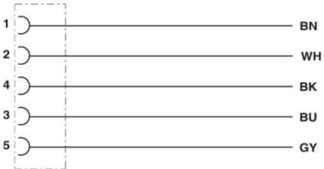
Contact assignment of M8 socket
