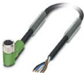
Sensor/actuator cable, 5-position, PUR halogen-free, black-gray RAL 7021, free cable end, on Socket angled M8, coding: B, cable length: 3 m
