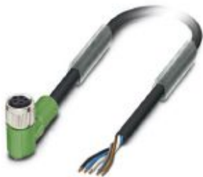
Sensor/actuator cable, 5-position, PUR halogen-free, black-gray RAL 7021, free cable end, on Socket angled M8, coding: B, cable length: 5 m
