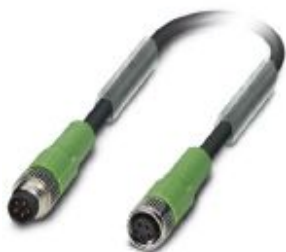
Sensor/actuator cable, 5-position, PUR halogen-free, black-gray RAL 7021, Plug straight M8, coding: B, on Socket straight M8, coding: B, cable length: 1.5 m
