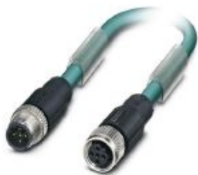
Bus system cable, PROFIBUS, 2-position, PUR/PVC, blue, shielded, Plug straight M12, coding: B, on Socket straight M12, coding: B, cable length: 15 m
