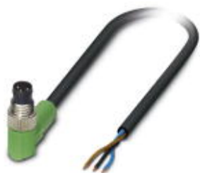
Sensor/actuator cable, 3-position, PVC, black RAL 9005, Plug angled M8, on free cable end, cable length: 5 m
