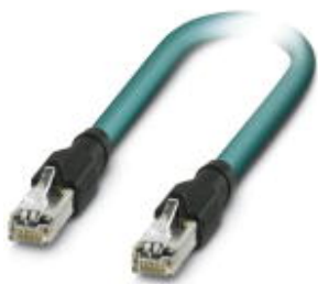
Patch cable, CAT5e, 4-pair, shielded, line, assembled with straight RJ45/IP20 heads at both ends, length: 10 m
