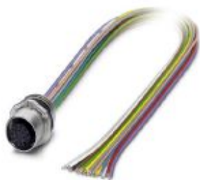
Sensor/actuator flush-type socket, 17-pos., stainless steel, front/screw mounting with M16 thread, with 0.5 m PVC litz wire, 17 x 0.14 mm 2
