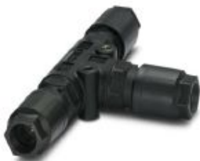
QUICKON T-distributor, black, 4+PE-pos., 1.0 mm 2 ... 2.5 mm 2 /690 V/20 A, for cable diameter of 9 mm ... 16 mm, with three QUICKON nuts
