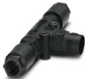
QUICKON T-distributor, black, 4+PE-pos., 1.0 mm 2 ... 2.5 mm 2 /690 V/20 A, for cable diameter of 6 mm ... 11 mm, with two QUICKON nuts
