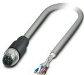
Bus system cable, CANopen®, DeviceNet™, 5-position, PVC, gray, shielded, Plug straight M12 SPEEDCON, coding: A, on free cable end, cable length: 2 m, Connector unshielded
