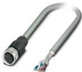
Bus system cable, CANopen®, DeviceNet™, 5-position, PVC, gray, shielded, free cable end, on Socket straight M12 SPEEDCON, coding: A, cable length: 10 m, Connector unshielded
