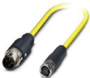
Sensor/actuator cable, 4-position, PVC, yellow, shielded, Plug straight M12, coding: A, on Socket straight M8, cable length: 1.5 m
