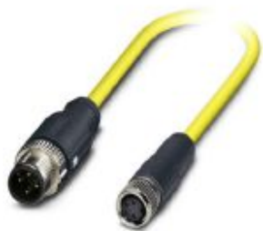
Sensor/actuator cable, 4-position, PVC, yellow, shielded, Plug straight M12, coding: A, on Socket straight M8, cable length: 0.5 m
