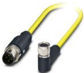
Sensor/actuator cable, 4-position, PVC, yellow, shielded, Plug straight M12, coding: A, on Socket angled M8, cable length: 1.5 m
