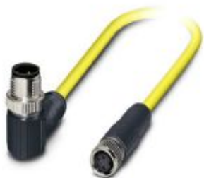
Sensor/actuator cable, 4-position, PVC, yellow, shielded, Plug angled M12, coding: A, on Socket straight M8, cable length: 1.5 m
