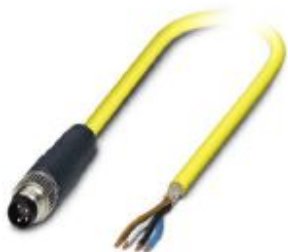
Sensor/actuator cable, 4-position, PVC, yellow, shielded, Plug straight M8, on free cable end, cable length: 5 m
