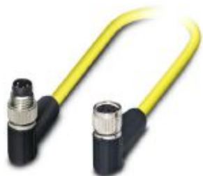
Sensor/actuator cable, 4-position, PVC, yellow, shielded, Plug angled M8, on Socket angled M8, cable length: 1.5 m
