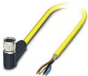
Sensor/actuator cable, 4-position, PVC, yellow, shielded, free cable end, on Socket angled M8, cable length: 10 m
