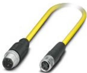
Sensor/actuator cable, 3-position, PVC, yellow, shielded, Plug straight M12, coding: A, on Socket straight M8, cable length: 0.5 m
