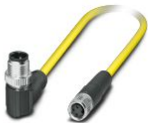
Sensor/actuator cable, 3-position, PVC, yellow, shielded, Plug angled M12, coding: A, on Socket straight M8, cable length: 1.5 m
