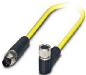
Sensor/actuator cable, 3-position, PVC, yellow, shielded, Plug straight M8, on Socket angled M8, cable length: 1.5 m
