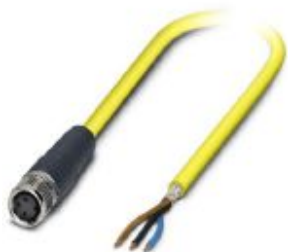
Sensor/actuator cable, 3-position, PVC, yellow, shielded, free cable end, on Socket straight M8, cable length: 2 m
