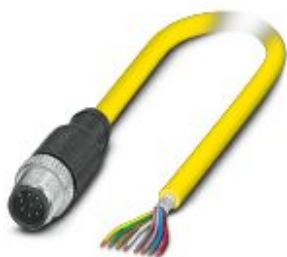
Sensor/actuator cable, 8-position, PVC, yellow, shielded, Plug straight M12, coding: A, on free cable end, cable length: 10 m
