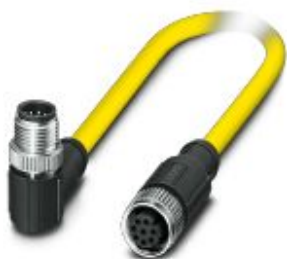
Sensor/actuator cable, 8-position, PVC, yellow, shielded, Plug angled M12, coding: A, on Socket straight M12, coding: A, cable length: 1.5 m
