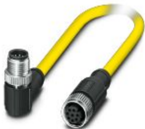
Sensor/actuator cable, 8-position, PVC, yellow, shielded, Plug angled M12, coding: A, on Socket straight M12, coding: A, cable length: 0.5 m
