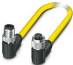
Sensor/actuator cable, 8-position, PVC, yellow, shielded, Plug angled M12, coding: A, on Socket angled M12, coding: A, cable length: 1.5 m
