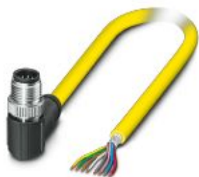
Sensor/actuator cable, 8-position, PVC, yellow, shielded, Plug angled M12, coding: A, on free cable end, cable length: 2 m
