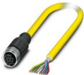
Sensor/actuator cable, 8-position, PVC, yellow, shielded, free cable end, on Socket straight M12, coding: A, cable length: 2 m
