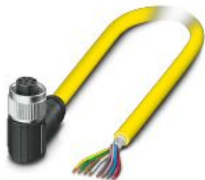
Sensor/actuator cable, 8-position, PVC, yellow, shielded, free cable end, on Socket angled M12, coding: A, cable length: 5 m
