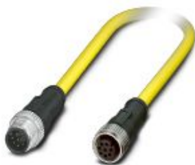
Sensor/actuator cable, 8-position, PVC, yellow, Plug straight M12, coding: A, on Socket straight M12, coding: A, cable length: 1.5 m
