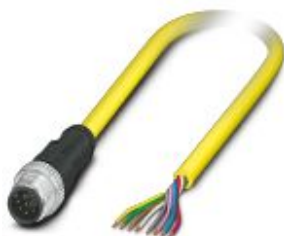
Sensor/actuator cable, 8-position, PVC, yellow, Plug straight M12, coding: A, on free cable end, cable length: 10 m
