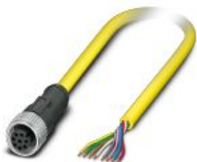
Sensor/actuator cable, 8-position, PVC, yellow, free cable end, on Socket straight M12, coding: A, cable length: 10 m
