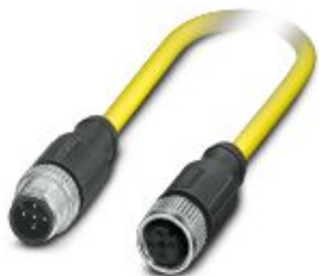
Sensor/actuator cable, 5-position, PVC, yellow, shielded, Plug straight M12, coding: A, on Socket straight M12, coding: A, cable length: 1.5 m
