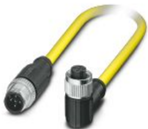
Sensor/actuator cable, 5-position, PVC, yellow, shielded, Plug straight M12, coding: A, on Socket angled M12, coding: A, cable length: 0.5 m
