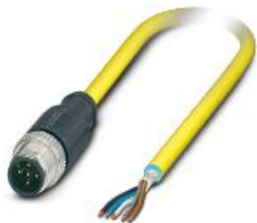
Sensor/actuator cable, 5-position, PVC, yellow, shielded, Plug straight M12, coding: A, on free cable end, cable length: 5 m
