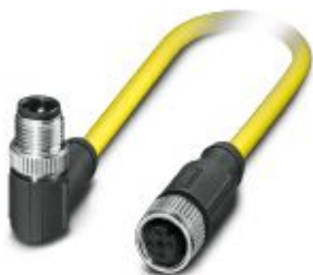
Sensor/actuator cable, 5-position, PVC, yellow, shielded, Plug angled M12, coding: A, on Socket straight M12, coding: A, cable length: 1.5 m
