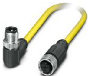
Sensor/actuator cable, 5-position, PVC, yellow, shielded, Plug angled M12, coding: A, on Socket straight M12, coding: A, cable length: 0.5 m
