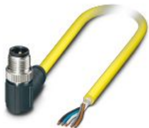
Sensor/actuator cable, 5-position, PVC, yellow, shielded, Plug angled M12, coding: A, on free cable end, cable length: 5 m
