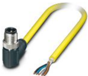
Sensor/actuator cable, 5-position, PVC, yellow, shielded, Plug angled M12, coding: A, on free cable end, cable length: 2 m
