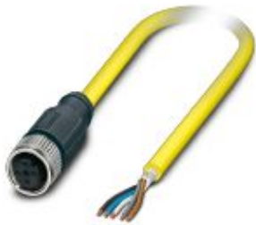
Sensor/actuator cable, 5-position, PVC, yellow, shielded, free cable end, on Socket straight M12, coding: A, cable length: 5 m
