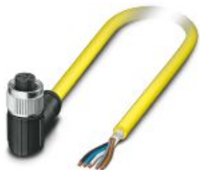
Sensor/actuator cable, 5-position, PVC, yellow, shielded, free cable end, on Socket angled M12, coding: A, cable length: 2 m
