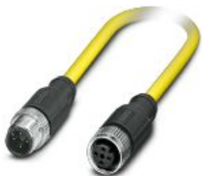
Sensor/actuator cable, 4-position, PVC, yellow, shielded, Plug straight M12, coding: A, on Socket straight M12, coding: A, cable length: 1.5 m
