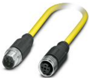
Sensor/actuator cable, 4-position, PVC, yellow, shielded, Plug straight M12, coding: A, on Socket straight M12, coding: A, cable length: 0.5 m
