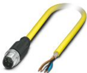
Sensor/actuator cable, 4-position, PVC, yellow, shielded, Plug straight M12, coding: A, on free cable end, cable length: 5 m
