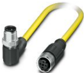
Sensor/actuator cable, 4-position, PVC, yellow, shielded, Plug angled M12, coding: A, on Socket straight M12, coding: A, cable length: 1.5 m
